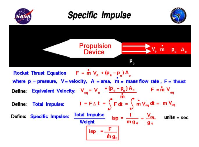
Thrust is the force which moves a rocket through the air. Thrust is generated by the rocket engine through the reaction of accelerating a mass of gas. The gas is accelerated to the rear and the rocket is accelerated in the opposite direction. To accelerate the gas, we need some kind of propulsion system. We will discuss the details of the propulsion system on some other pages. For right now, let us just think of the propulsion system as some machine which accelerates a gas.
